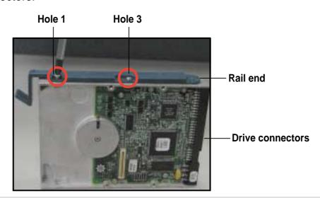
3. Attach **Rail 2** to the other side of the drive as shown. The rail end should be on the side of the drive connectors.
